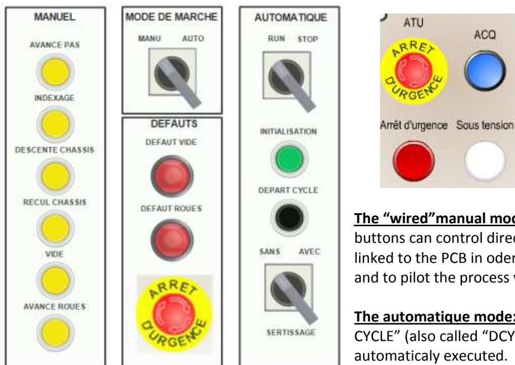
**The “wired” manual mode:** used for tests. The push buttons can control directly each actuator and are not linked to the PCB in order to lower the number of inputs and to pilot the process without microcontroller.
