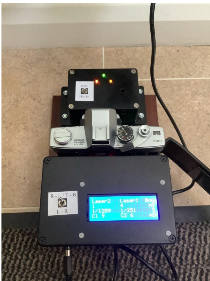
Three laser design for horizontal or vertical shutters. Switch toggles horizontal or vertical Laser.
