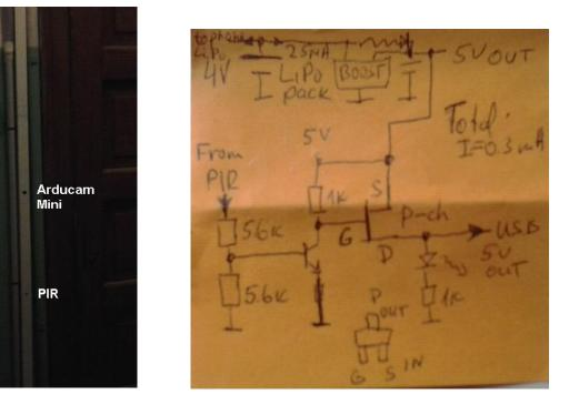
PIR-controlled power circuit idea was taken from <u>https://www.opensmartcam.com</u> and my instructable <u>http://www.instructables.com/id/GSM-Android-phone-as-HD-outdoor-webcam/</u>
