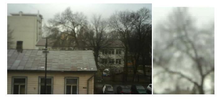
Tested Arducam in low-light conditions – stairways illuminated by a 7W fluorescent lamp. One sees camera dark noise. As exposition is long, there is motional blur of moving objects . At same conditions Samsung Galaxy tab camera image was not darker because it has even smaller lens opening . It could help to use a larger diameter lens to collect more light like used in traditional CCD security cameras. NIR illumination is actually needed!
