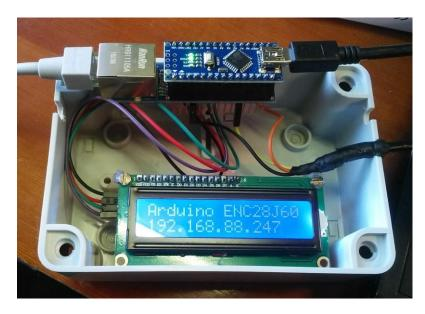
This version has the quickest and easiest assembly of all. One needs to file holes for cables and to glue LCD. That's it. But in order to change Eth cable or USB cable one needs to unscrew the box lid which is an easy work. Nice dust protection.
