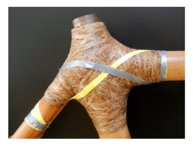
**2nd Wrap Set (latches front and rear triangles together and adds some lateral stiffness)** Anchor your first piece of fiber on the TT and spiral counter clockwise (viewed from the front) toward the rear of the frame, loop once around the bottom ST and continue to spiral toward the right side SS. Anchor at LL.
