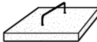
Concrete lid with metal handle
