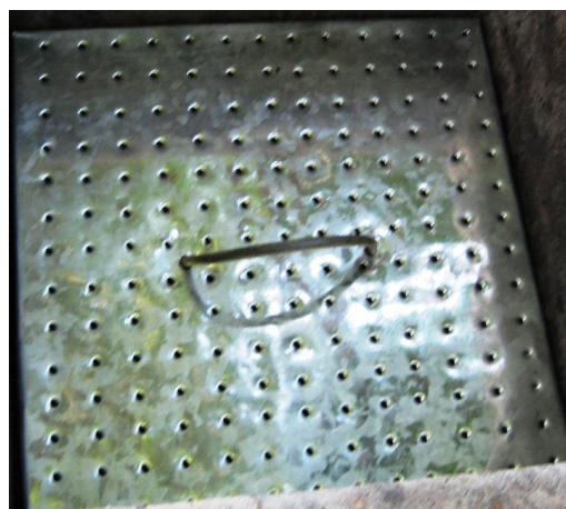
Holes should be 3mm diameter, 2.5 cm (1") apart.
