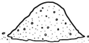
Sand and gravel (mixed or separate) suitable for filtration material
