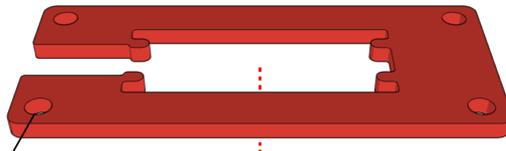
To help with assembly, insert a temporary screw into one of the holes from the bottom. Keep the layers together by placing each layer onto that screw.
