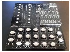
22. Solder all 3 S&T GeoTronics 3Segments (Custom Plus/Minus).
