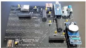
25. Solder the Speaker and MP3 Player/SD card making sure to respect orientation AND keeping as high up on the PCB because the GPS on the other side will need to be flush with PCB to fit properly.
