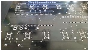
8. Cut 2 strips of female pin connectors and solder them to Arduino Nano location on back of PCB.
