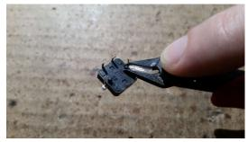
13. Insert, then solder all 13 Lighted push buttons, making sure all the red dots (Cathode) are on the left side. Once all buttons are inserted, I power up the Arduino via its USB port to test that all 19 button LEDs turn on BEFORE I solder them...
