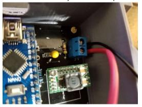
9. Screw a Jumper wire to 9V side of Blue Screw Terminal and solder the other end to the available pin on On/Off Rocker switch.
