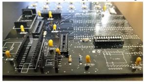
19. Solder the Reed Relay, making sure to respect orientation.
