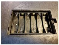
8. Screw the Black wire from battery box in the Gnd position of Blue Screw Terminal and Solder the Red wire from battery box to either pins on On/off Rocker switch.
