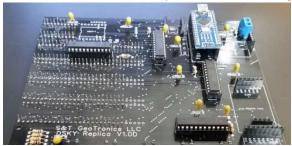
24. Insert the IMU, RTC, Buck, Arduino Nano and Line Leveler.
