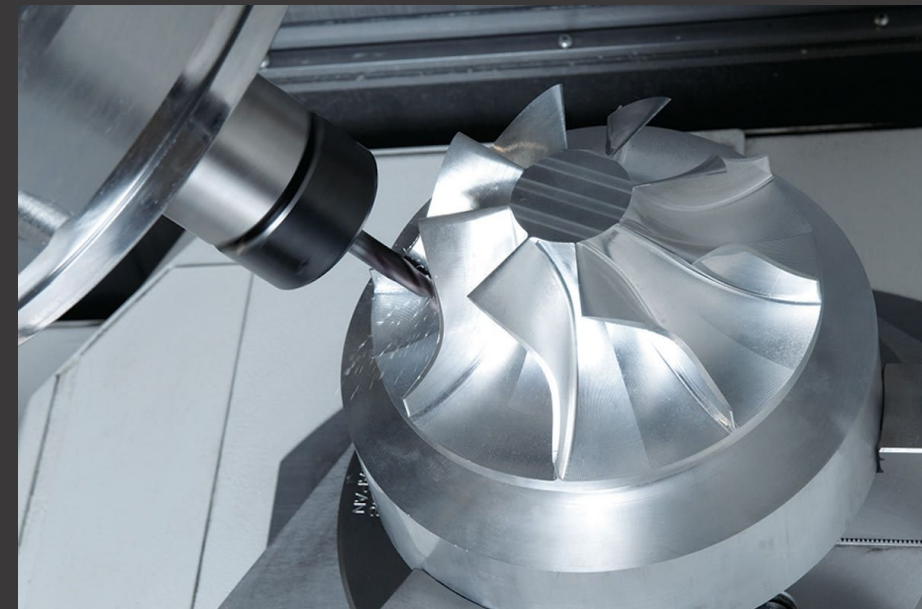
a 5-axis mill can cut more complex geometry
