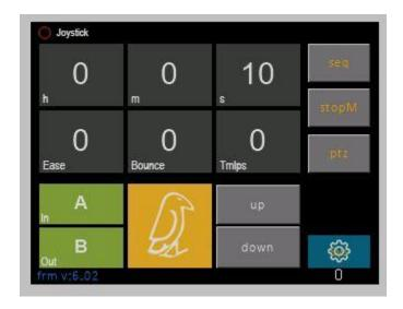
When you first power on the controller you will be taken to the home menu which provides all the basic controls for A-B programmed moves.
