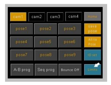
Each camera system and lens arrangement will require different limits to be set on the DB3 head. This is the case regardless of whether you are using the system in WIFI or wired VISCA mode. We can set those limits using the **[Limits]** button on the PTZ menu.
