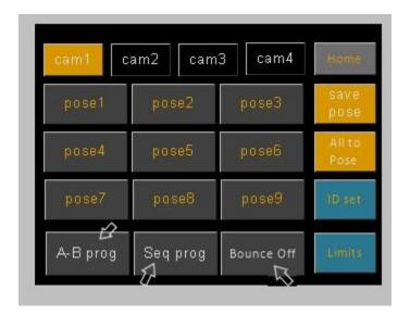
At the bottom of the PTZ menu you will see three buttons: **[A-B prog]** [ **Seq prog]** and **[Bounce]** this is a new feature on V6. Essentially these buttons allow you to call your pre-programmed A-B move and sequencer moves as though they were PTZ presets. Bounce can be either on or off for the moves. Essentially the system utilizes presets 15 and 16 for this purpose which allows you to start either of the programmed moves from OBS or your PTZ controller using VISCA commands.
