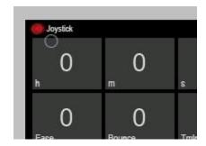
If you are using the PTZplus controller you can also use the joysticks on the controller to move the system to your required in and out positions. To do this you must first press the small button on top of the large 3 axis joystick. On the display you should see the small dot next to the word "joystick" at the top left corner turn solid red.
