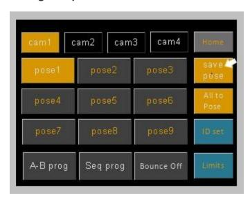
Poses or Presets are recorded positions for all axes on your system which can be recalled with the tap of a button. Poses saved using the WIFI controller can also be recalled from OBS using the VISCA connection however vMix does not use the memory slots on the head but keeps its own record of the positions and will therefore not recognise presets saved from the WIFI controller.
