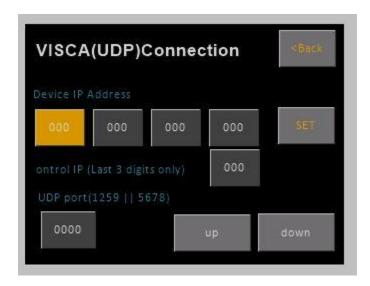
This is where we set the DB3 head network IP address. When using the system wired over VISCA each PTZ head must have its own unique IP address. Any number of heads can be controlled with OBS or vMix provided each has its own unique address. When you first select this option you will see a splash screen warning you that only one head should be powered up when performing this task. If two or more heads are powered up they will all be stamped with the same IP address!
