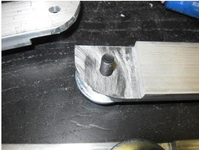
Washer and bolt installed in thigh support
