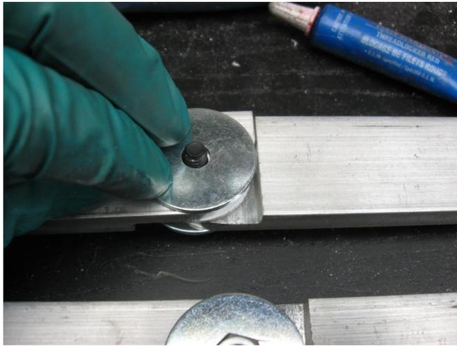
Inner fender washer installed
