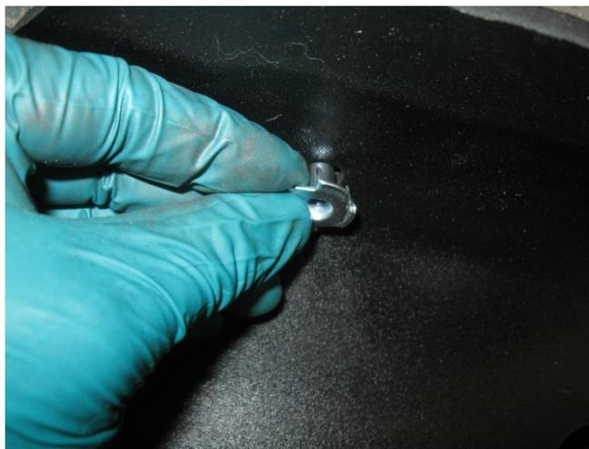
Placing Tee Nut in Sintra
