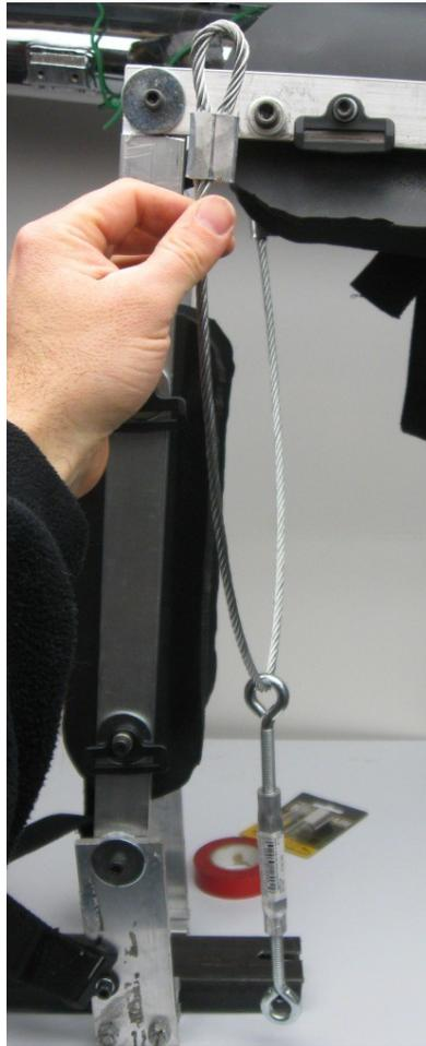
Installing cable and turnbuckle assembly
