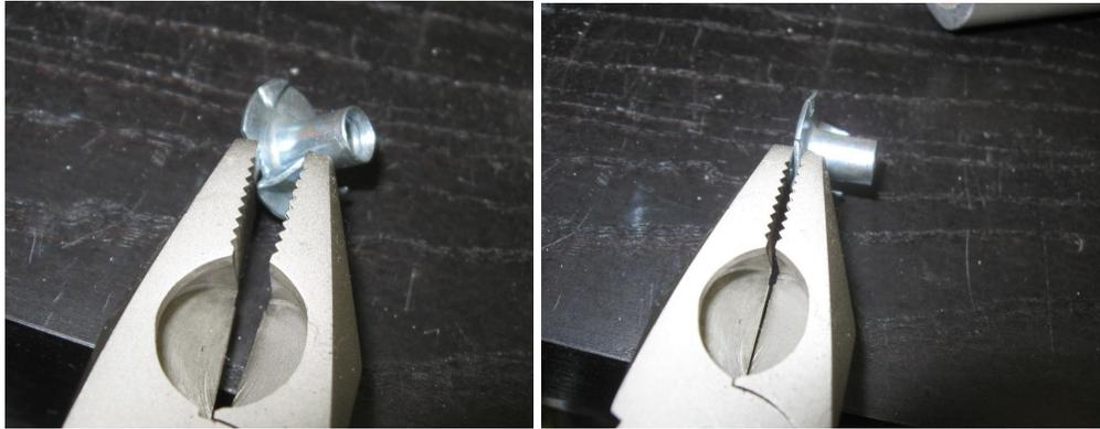
Grip the Tee Nut Prongs with pliers to flatten
