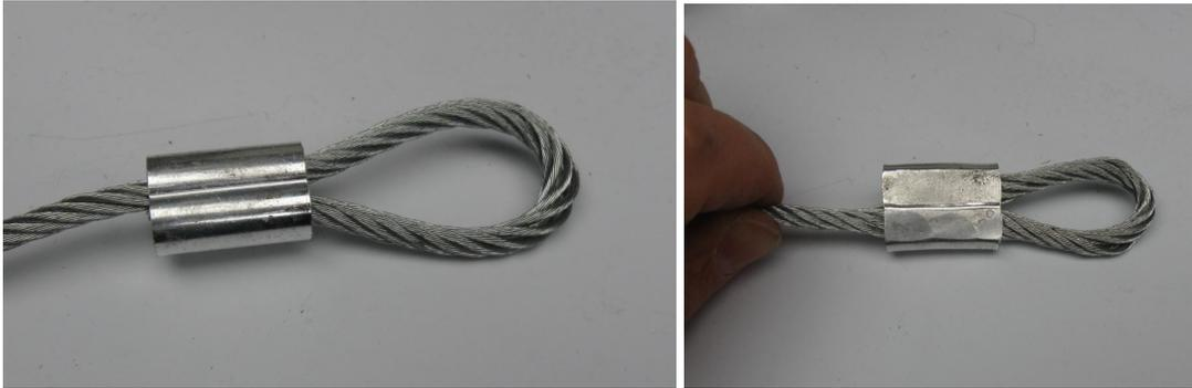
Sleeve shown installed then flattened
