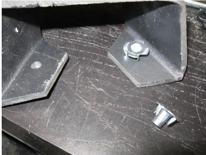
Placing Tee Nuts in toe clips
