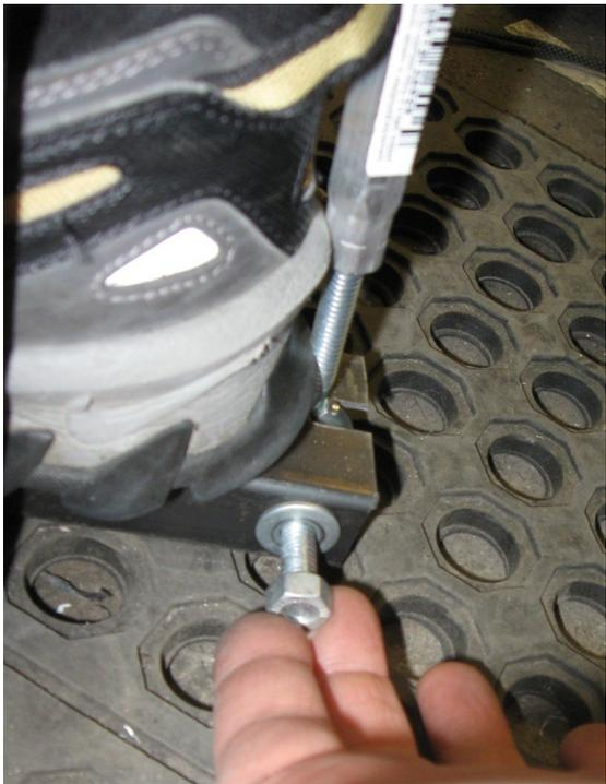
Installing the Achilles (heel) bolt
