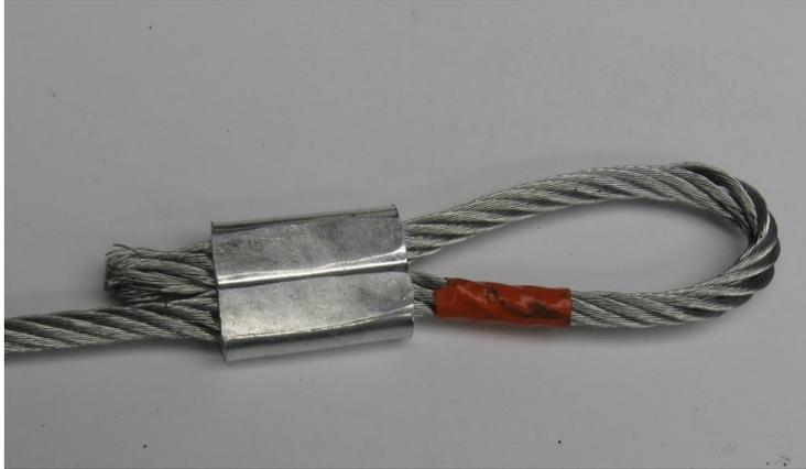
Incorrect cable loop with frayed cable.
