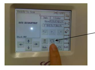
Hit this trace button with the foot up to make the machine move in a rectangle above the area it will be embroidering. If this box is too big hit the size button above to scale everything down to 90%. If it goes off the top or bottom of the ribbon readjust using the arrows and trace again.
