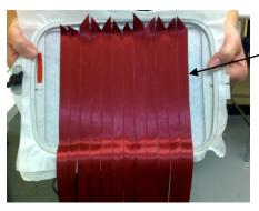
The ribbons do not extend outside of the printable area, and the excess is on the outside so it hangs down off the machine.
