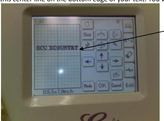
Text is not centered. Use the down arrow to align the bottom of the box with the center horizontal line.
