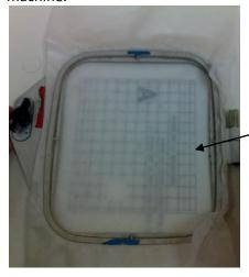
The grid is important for aligning the ribbon and seeing where the printable area of your embroidery machine is.
