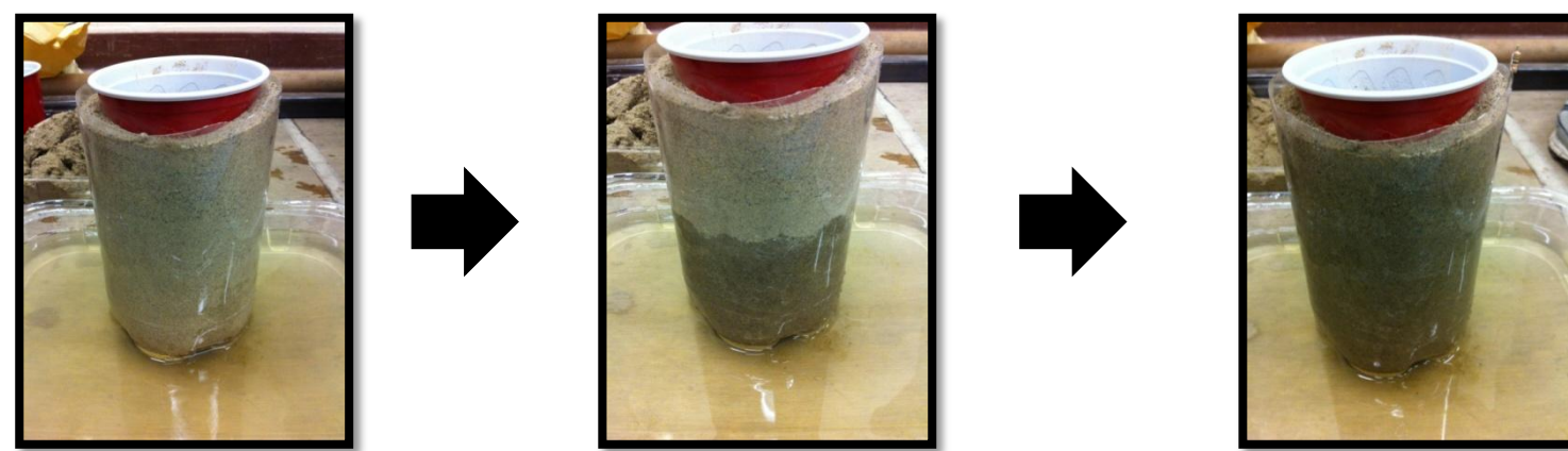
Fine grain sand in a vertical container easily saturates from a shallow pool of water within a few seconds
