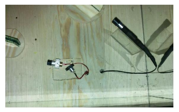
Below is a photo ofmains connections. All setup is activated by flipping the red switch. Adjustable power supply is set to 24V for driving the fog generator.
