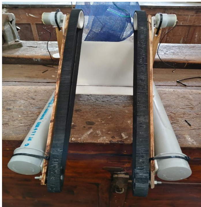
Figure 5.2 Installation of belt drive
