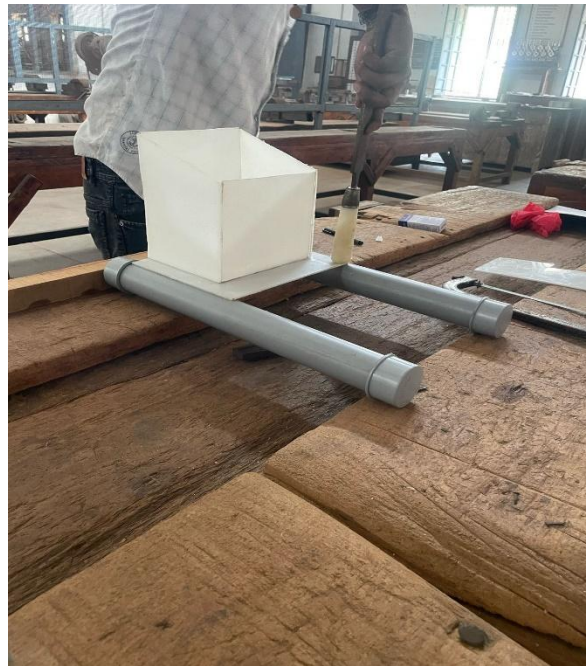
Figure 5.1 Base frame and collecting tank
