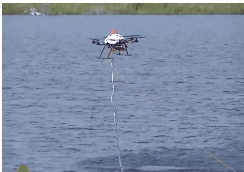
Figure 1.4 Drone-Based Water Monitoring
