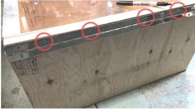
8. Open the hinge and center the thin strip of plywood against it. Mark and pre-drill a few screw holes in the strip. The screws will be near the edge of the wood so pilot holes are important to prevent tear-out. A 1.5in wide hinge works well for  $\frac{1}{8}$ in polycarbonate, but for  $\frac{1}{4}$ in thick polycarbonate a 2in wide hinge will center the holes better.
