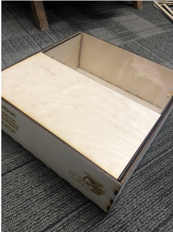
Figure 14: Laser cut wooden box with uncut wooden panel and acrylic pane for lid.
