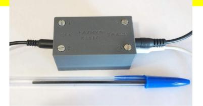
There is a side labeled KEY where you have to insert the jack of the paddle/key The side labeled TRANS is for the transceiver jack. In the same side you have the microUSB connector for the power suply.
