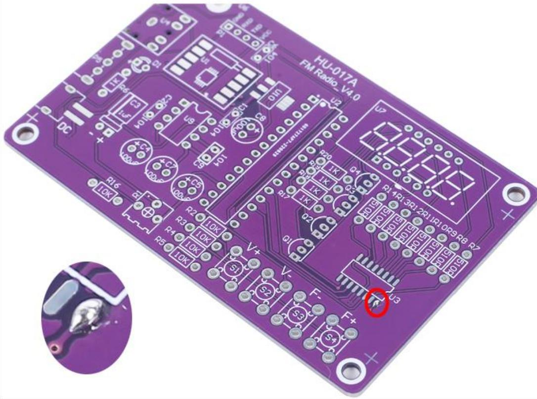
Step 4: Connect others pads on 74HC595D to pads on PCB by tin and soldering iron.
