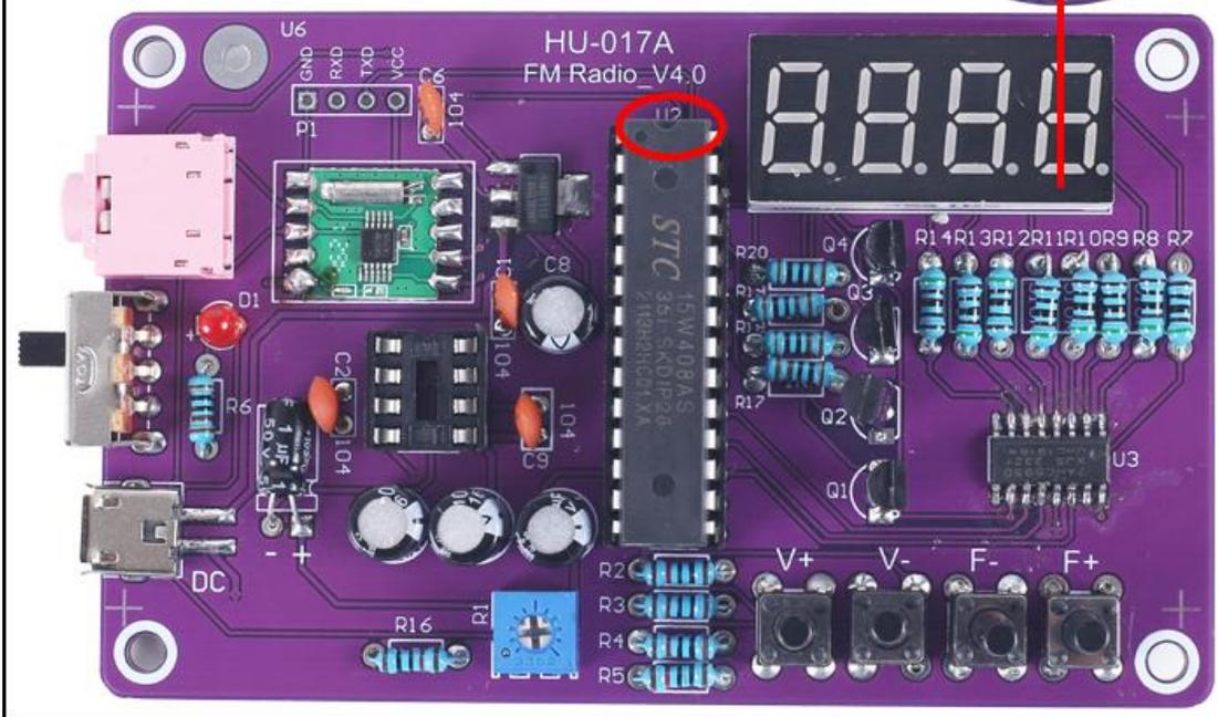
Step 24: Install 1pcs DIP-8 TDA2822M Amplifier at U9. There is a gap mark on one end of the IC and there is a gap mark on DIP-8 IC Socket where the IC can place on. These two marks are corresponding to each other and are used to specify the installation direction of the IC.
