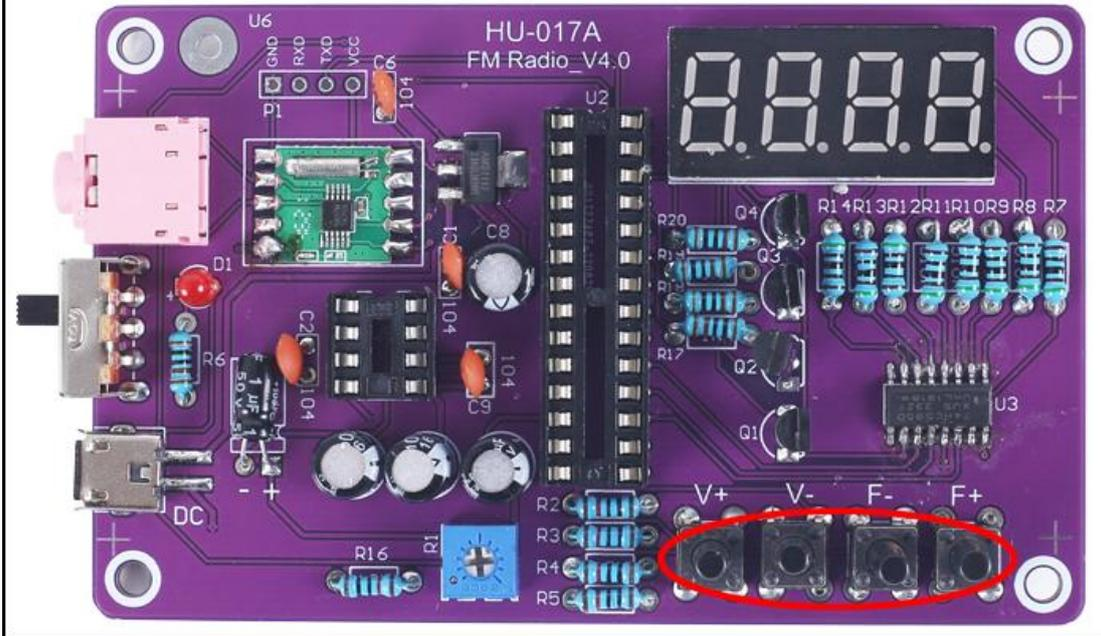
Step 23: Install 1pcs DIP-28 STC15W404AS MCU at U2. There is a gap mark on one end of the IC and there is a gap mark on DIP-28 IC Socket where the IC can place on. These two marks are corresponding to each other and are used to specify the installation direction of the IC.
