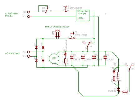
separate circuits used for loading ammunition, laser targeting systems and more, the core Coilgun circuit has been expanded upon. A few ways in which we can see that this system has improved upon the previous circuit is the fly back diode as mentioned earlier, and a bulb which acts as a charging resistor. This has been implemented in order to more safely allow the charging capacitors to dissipate energy (an
