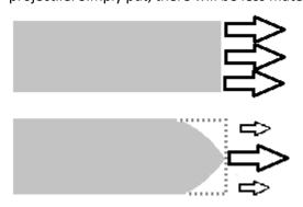
paramagnetic tip on the bullet which does not interfere with the magnetic flux (allowing the metallic section to remain entirely flat and cylindrical), or simply to be cautious of how much you grind away — making the bullet only slightly rounded. It is questionable which would be more efficient, since the tipped projectile would have greater magnetic flux but more dead weight, while the rounded one would have a reduced magnetic flux but lower mass.
