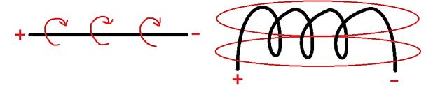
the core, and the total number of turns of wire. It is also worth noting that too many turns will increase the resistance of the circuit and lower the current, meaning that an optimum number of turns must be found in order to maximise strength.
