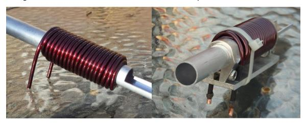
I also made a hole through the tube and clamp in order to fit the infrared detection system later on, using a drill press. In order to avoid damage to the enamel layer, I filed all edges that I cut, and wrapped electrical tape around particularly prone areas. This can be removed if it cannot handle the high temperatures, but having it on while I fed the wire through prevented any scratching.
