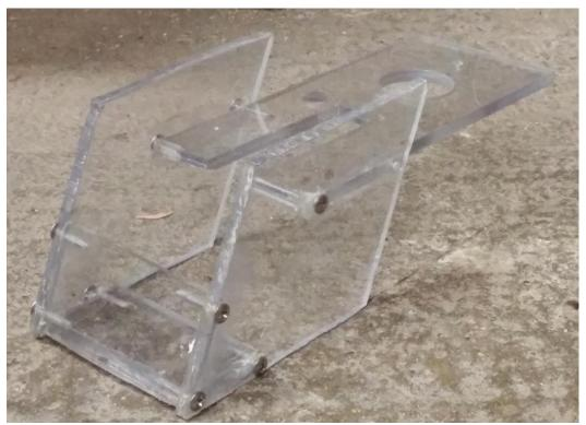
I had less trouble this time with the polycarbonate because I ensured that I drilled long enough pilot holes and held all of the parts in position with epoxy before screwing them together. This did result in a slight loss of aesthetic appeal since the epoxy ruined the clear transparent effect of the polycarbonate, but this was not at all a concern for a prototype.
