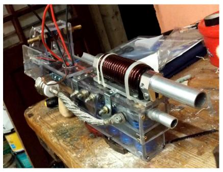
long. Given that it was steel, its mass was simply too high. The force required give the projectile a reasonable acceleration would have to be massive, and I had not fully considered this because I was more concerned with the fact that a large projectile would take advantage of all of the magnetic flux in that area.
