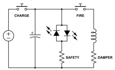
This is simply a charging circuit at the left, to charge the capacitor, and then a trigger which directs the energy stored in the capacitor through the coil. A capacitor is used rather than a battery because a Coilgun needs a short but very high supply of power, which can be provided by a fast-discharging capacitor (a battery would be lower-power and discharge much more slowly). It also features a
