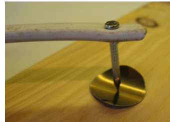
Put the disc on a bit of scrap wood and hold a nail in the middle
