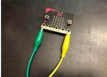
I made music (song of Jingle Bells) and light beneath the snow globe by using Microbit and a headphone. First, I made code in Microsoft Makecode. I uploaded the code into my Microbit. I connected to the headphone using two alligator clips. One is plugged into Pin 0 (P0) and the other into the ground. On the other side of alligator clips, I connected both of them into the headphone jack in the headphone. Automatically, the music is on.
