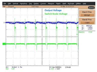
Figure 6. Ripple Voltage for 1600 μF Capacitance
