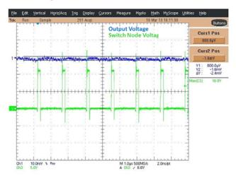
Figure 7. Ripple Voltage for 3200  $\mu$ F Capacitance
