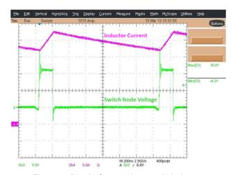
Figure 4. Ripple Current for 0.3 µH Inductor
