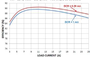
Figure 9. Effect of Inductor DCR on Efficiency
