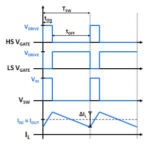
Figure 2. Synchronous Buck Converter Waveforms
