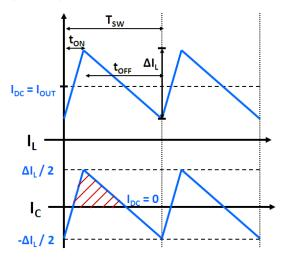
Figure 3. Inductor and Capacitor Current
