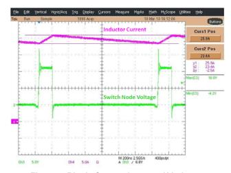
Figure 5. Ripple Current for 0.82  $\mu H$  Inductor
