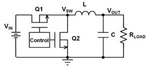
Figure 1. Synchronous Buck Converter
