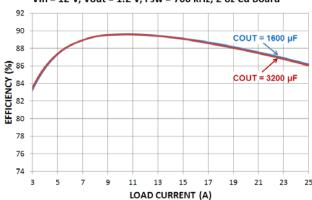
Figure 8. Effect of Capacitance on Efficiency
