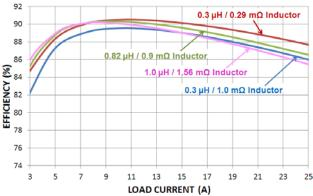
Figure 10. Effect of Inductance on Efficiency
