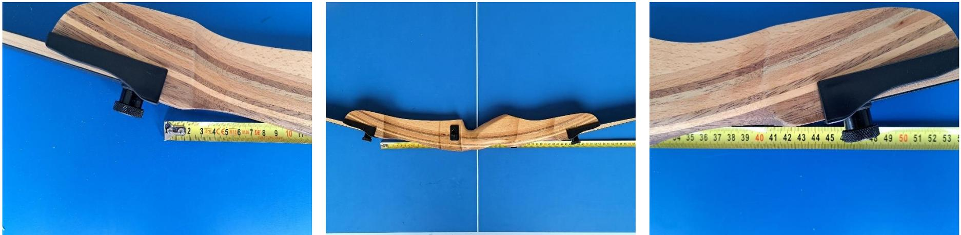
As shown in the photo's the distance between the points on which the handle will rest are 44 cm apart.
