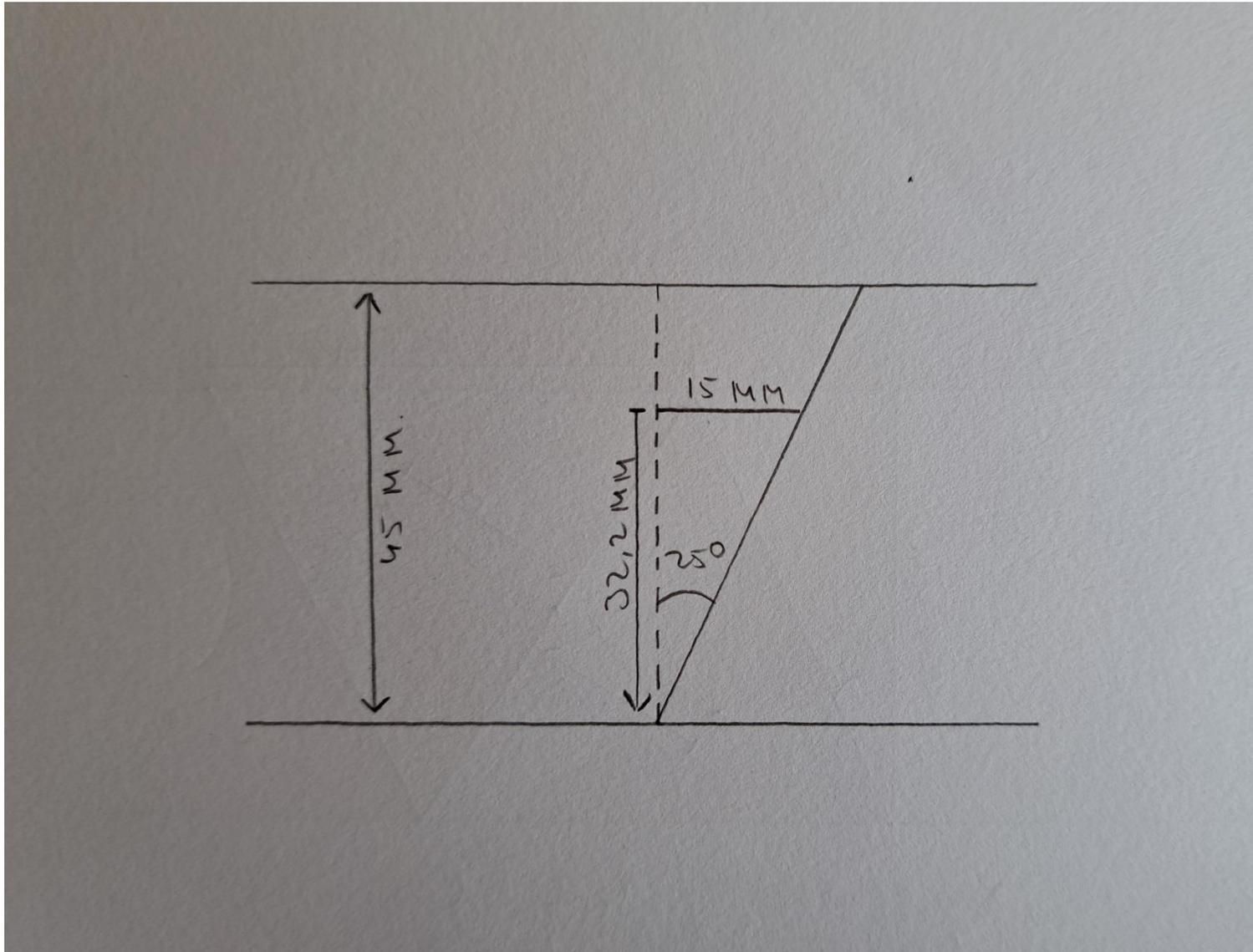
I: Measurement for drawing out the dowel holes for the support blocks
