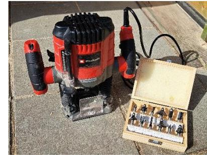
Q: Router drill with drill bits
