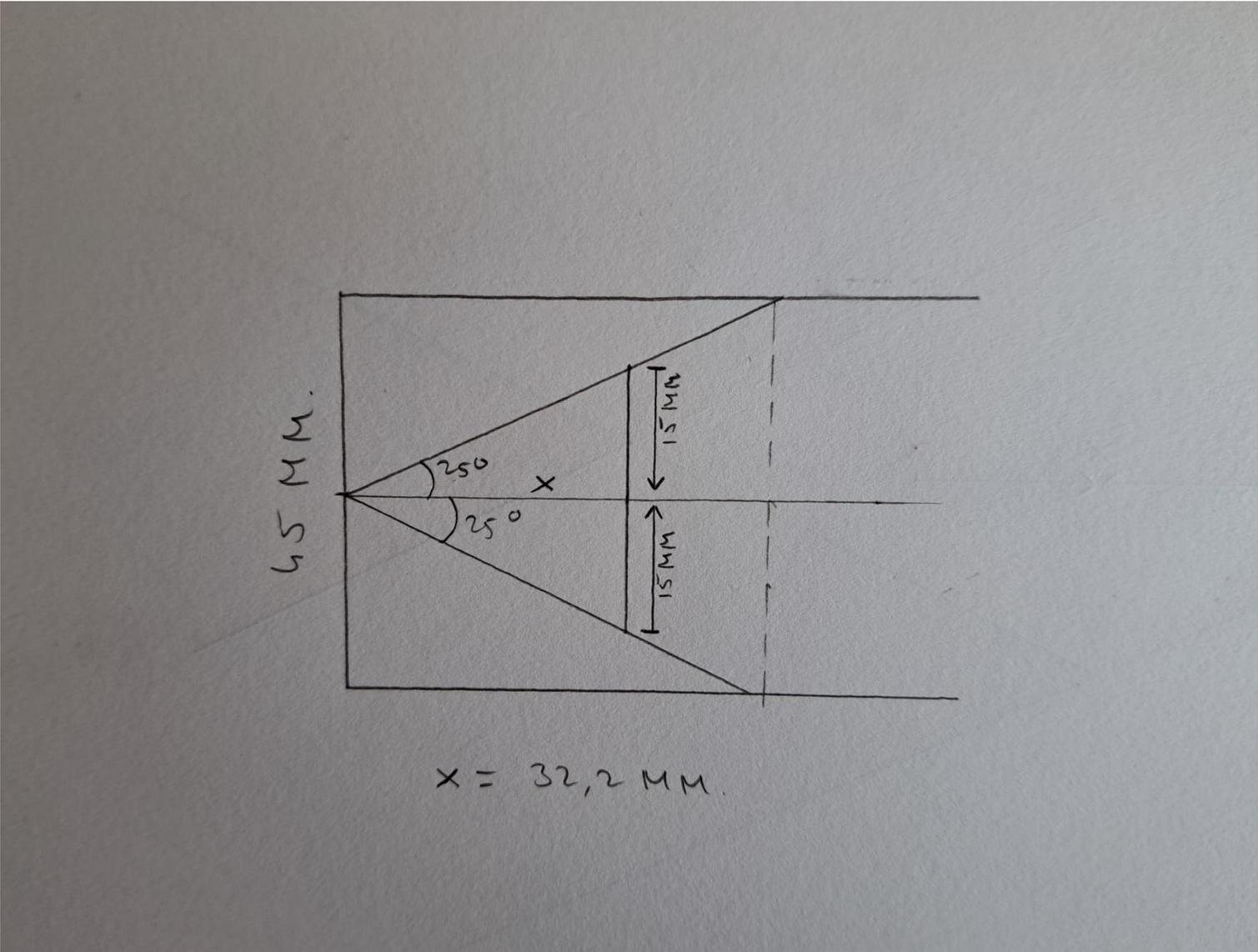
H: Measurements to determine the 25° angle
