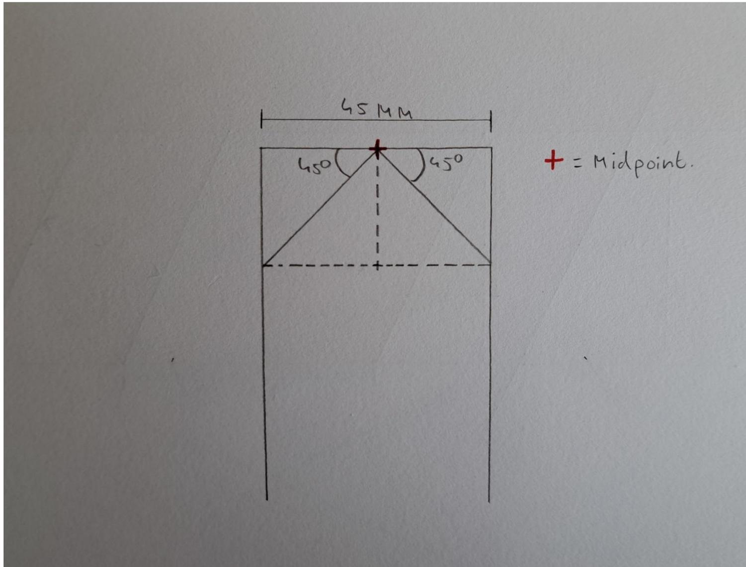
E: Sketch of the guidelines used for sawing and routing
