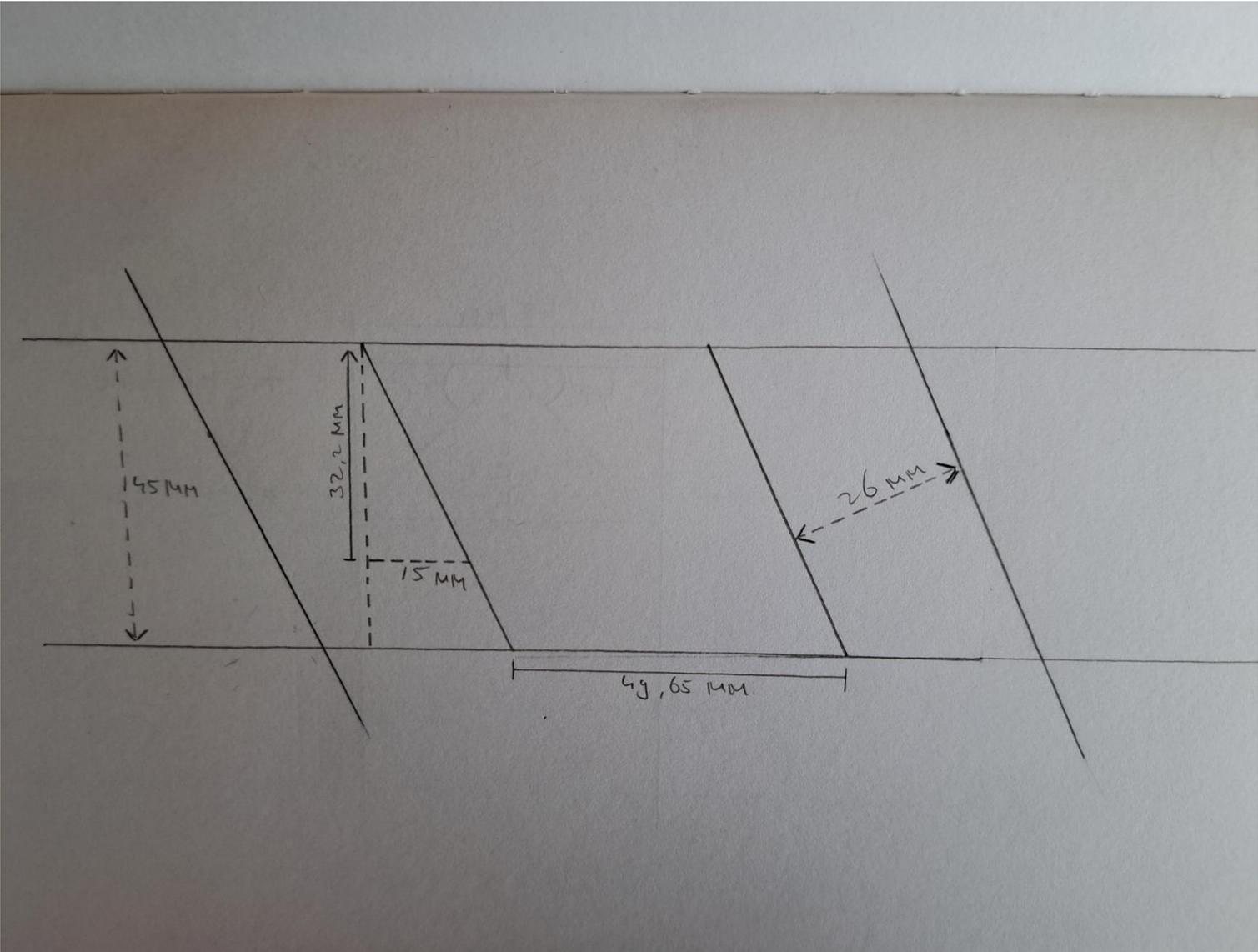
F: Sketch of the position of the dowels in the lower joint
