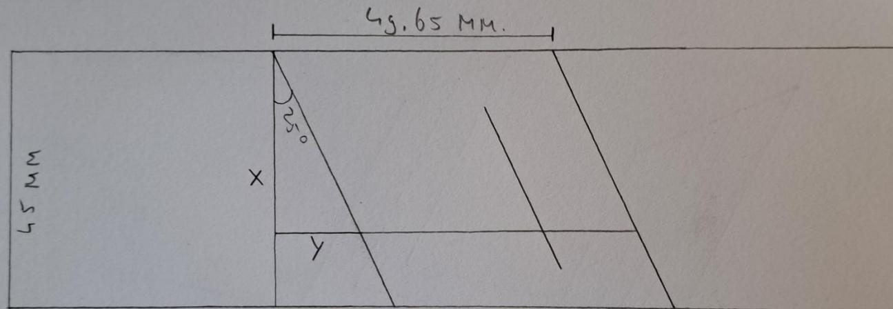
$$y \rightarrow \underline{15 \text{ MM}} \Rightarrow x = \frac{15}{\tan(25)} = \underline{32,2 \text{ MM}}$$
