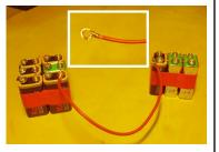
The last block to be connected in series needs a longer cable to cover the gap (because the magnet goes in between).
