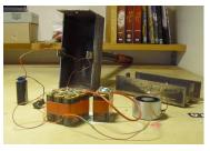
The complete circuit waiting to be packed. From left to right: The battery for the relay, the relay, the power unit (27V) and the electro magnet.
