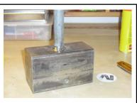
Like every good project, this too started off on the designing table. The original plans are a bit crude, though some ideas (copper wire, meassures) were already sketched out. See the included PDF file for a more refined layout. The metal used here is steel (3mm), bent to specifications (see PDF file).
