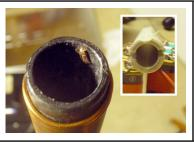
To keep it tight, bend the wire to the internal wall.
