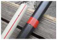
This is the hole **opposite** to the switch, seen before. To also keep the plastic tube from sliding inside the handle, but keeping it at the same time retractable in case of repair, I thought of making a channel, back and front. The hole on the plastic outlines the depth needed.
