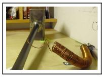
I put the pre-bent wire into the starting hole as deep as the plastic tube inside allowed, thus blocking it from escaping. With a (real) hammer, I bent the wire tight towards the handle's wall, then putt the loops on the handle and tightened them to the bottom. There the wire was cut and fixed to the bottom hole.
