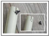
This micro switch actually has got four legs, but we need just two for our cables. One leg goes into the notch, for the second leg we need to drill another hole.
