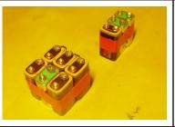
The batteries are bundled in 3x3 blocks, they are separated to leave a center space for the electro magnet. The batteries in each block are connected in paralleles. This way the Amperes are rising – thus the power of the electro magnet.
