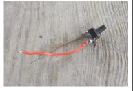
The two operating legs connected to wiring.
