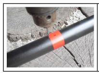
Let's see how we can fix the copper wire. How about providing a start and an end hole on the handle – like this the wire won't slide up or down, and is kept from unwinding itself, too.
