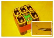
To get a higher voltage, the blocks are now connected in series. The little loop in the small picture connects minuses (3) of one block with the pluses (3) of the second block.
