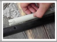
The place for the switch was marked before. The notch (rather than channel) allows me to bring the cables to the micro switch, which will "sit" on the plastic tube. Switch and copper starter are 180 degrees opposite to each other.
