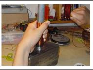
Then it's just pure handwork – turn the hammer and try to keep the wire as snuggly to the handle's wall as possible. At that moment I had no plan yet how to keep the wire fixed to the handle.
