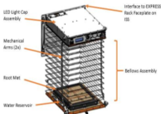
Figure 2. CAD model of Veggie, built by ORBITEC Technologies, Inc., primarily focused on the demonstration of successful food production in microgravity (image credit: ORBITEC).
