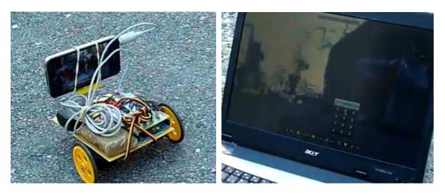
Dual frequency DTMF method is quite reliable and there exists a specialized decoder chip. DTMF chip is read out by Arduino board that controls servos.
