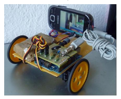
First version was to use single frequency tones 700, 800, 900, 1000, 1100, 1200 Hz. The tones were recorded by *Cooledit* as wave files 1 s long. Skype can transmit tones well in this range. Arduino had a program that counts frequency.
