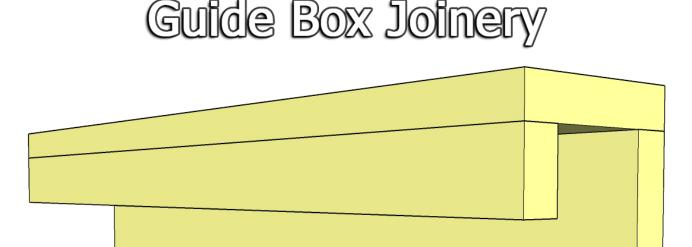
The only trick to watch with the Guide Box is **NOT** to add glue to the front face as you will need to remove it to screw the cleat to the wall. Space your pocket holes to give you room to drill the mounting holes in between.
