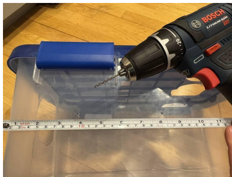
Drill two wire holes on each side roughly halfway up the wall, then thread the wire into a D shape.
