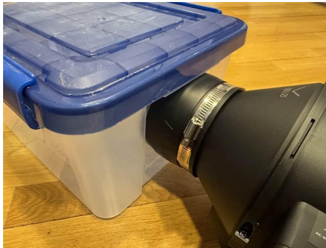
The rubber coupler joining the H4 discharge to the tote wall, worm clamp snugged.
