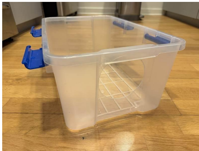
4" fan hole in the end wall, as high as the lid allows.
