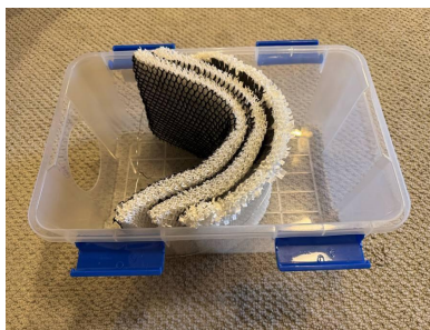
Cut each wick loop in half, stand the halves inside the wire, and check that the lid vents stay clear of the last wick.
