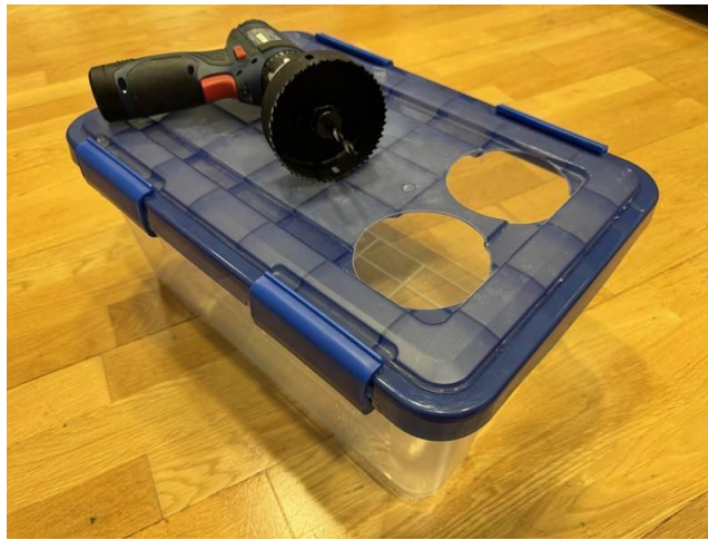
Two 3.5" vent holes in the lid, at the end opposite the fan.
