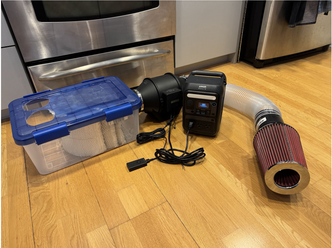
The complete v3 system: cooler tote, CLOUDLINE H4 fan, Anker SOLIX C300, dust collection hose, cone intake filter.
