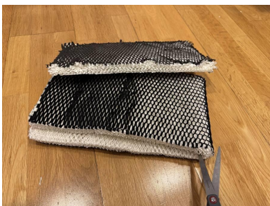
Cut each wick loop in half, stand the halves inside the wire, and check that the lid vents stay clear of the last wick.
