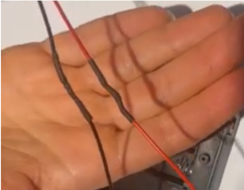
Photo 1.2: Visual inspection of heat-shrink tubing and solder joints (battery holder and PCB).
