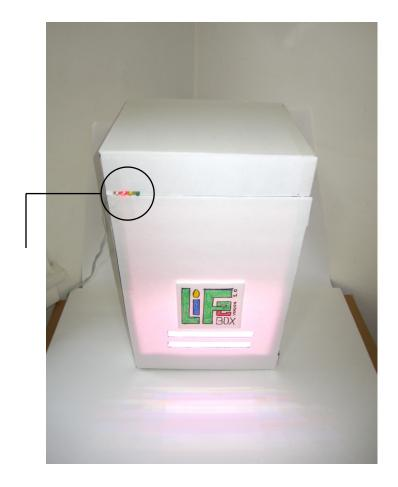
when all conditions are optimal (sun, water, temperature) The Life-Box stays lit green indicating perfect health. if either of the sensors are triggered the corresponding light comes on (sun>yellow, water>blue, temperature>red) and notifies the user to take action.
