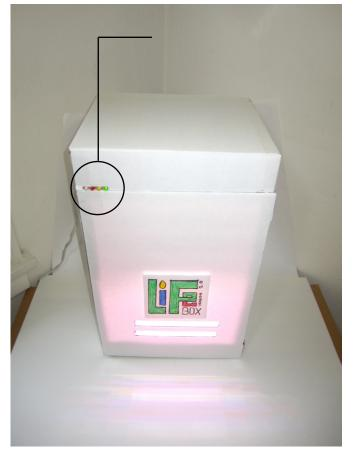
when all conditions are optimal (sun, water, temperature) The LifeBox stays lit green indicating perfect health. if either of the sensors are triggered the corresponding light comes on (sun>yellow, water>blue, temperature>red) and notifies the user to take action.
