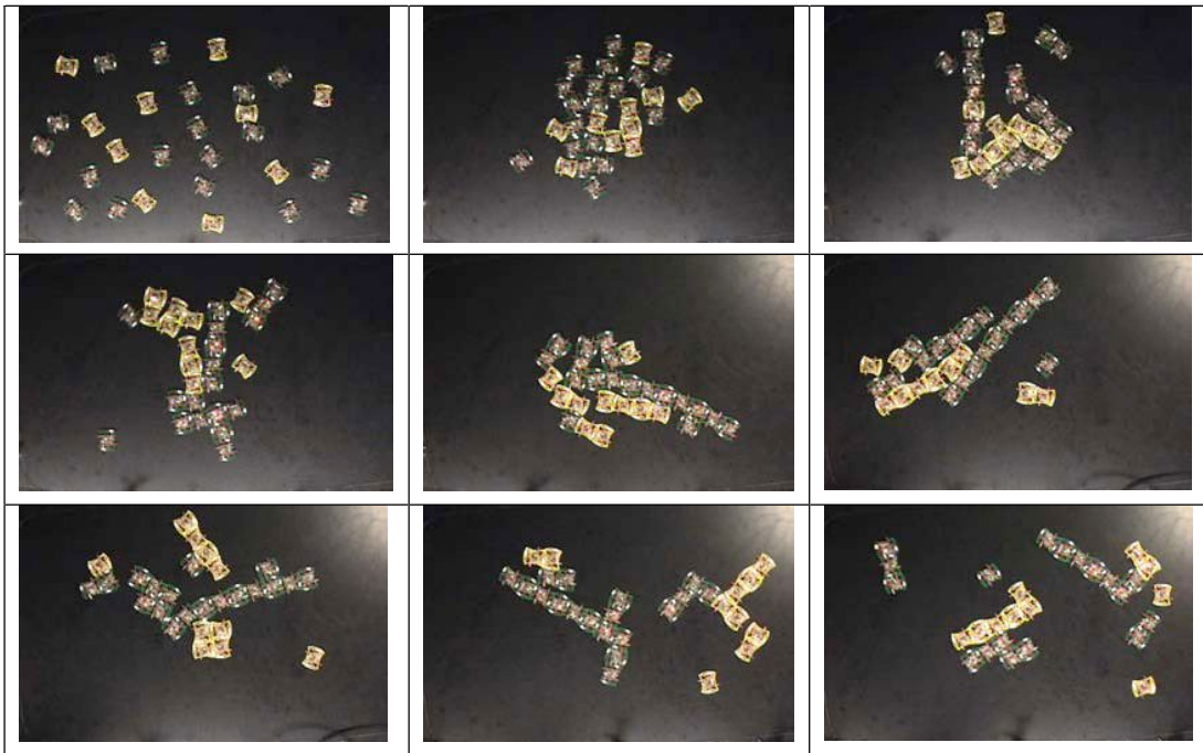
Figure 6-23 Screenshots from a line formation experiment. Series proceeds from left to right, top to bottom. The final state is seen in the bottom-most right hand picture. A number of different polymer chains can be seen to have grown.
