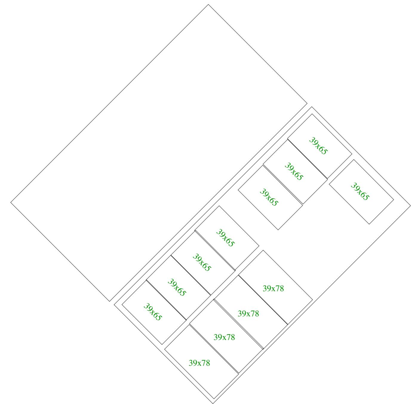
ROOF FLATTENED TO SHOW PANELS AT ORIGINAL ASPECT RATIO
